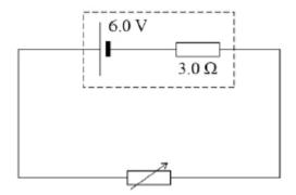
How much electrical energy is converted into thermal energy within the cell in 1 minute?
