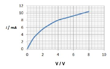
What is the resistance of the filament when the potential difference (pd) across it is 4.0 V?
