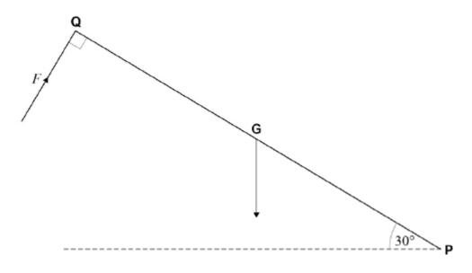
What force, F, acting perpendicular to  $\mathbf{QP}$  as shown, is required to hold the bonnet at 30° to the horizontal?
